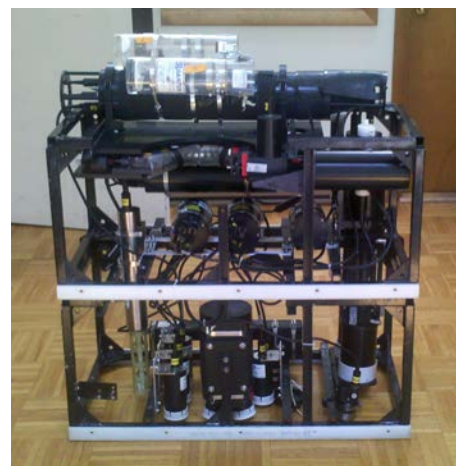
Figure 5.16: Inherent optical property instrument package deployed during SABOR.
