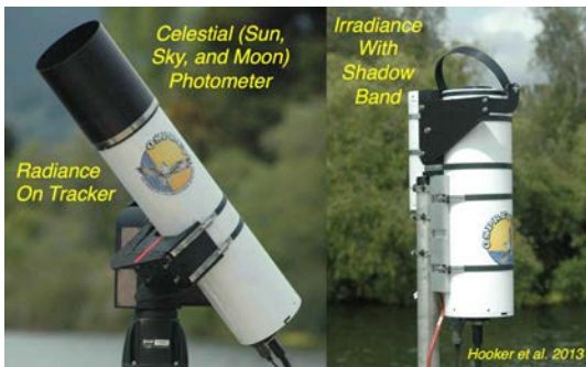
Figure 3.13: An OSPREy radiance & irradiance dyad deployed at a lake in 2013.
